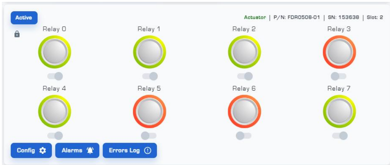
Figure 4: View of the output relay card display page in the device's user interface.
