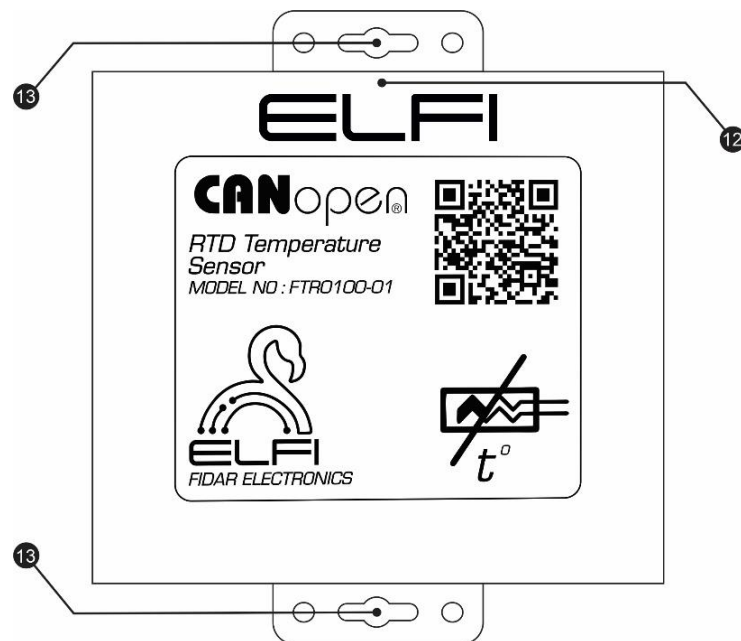
Figure 3: Front view of a PT100 Temperature Node
