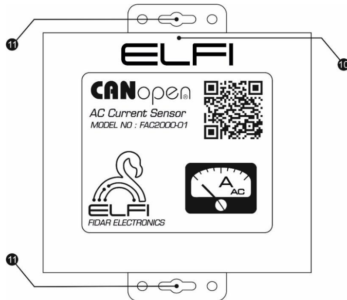
Figure 3: Front view of a single-channel AC Node
