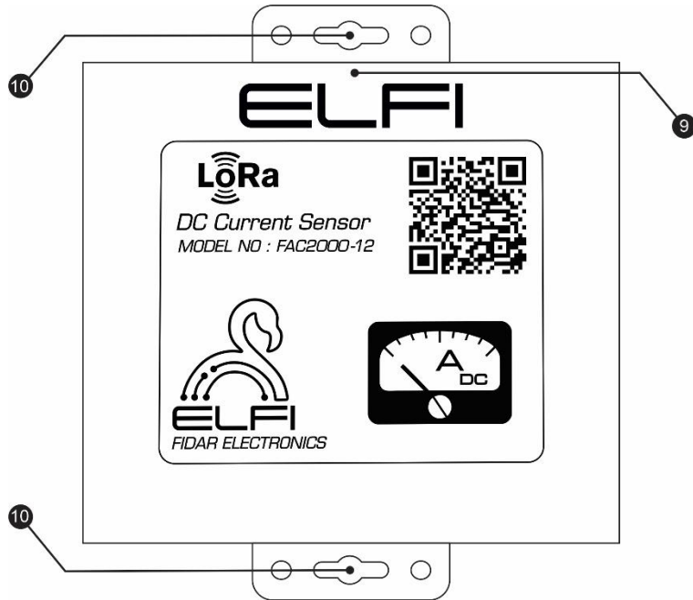
Figure 3: Front view of a wireless single-channel DC node
