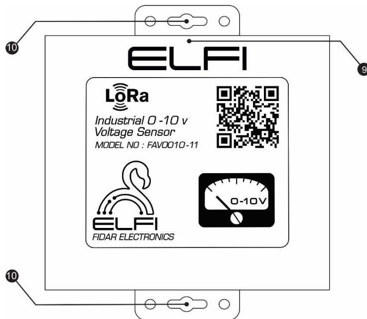
Figure 3: Front view of a Wireless single-channel 0-10 volt DC node
