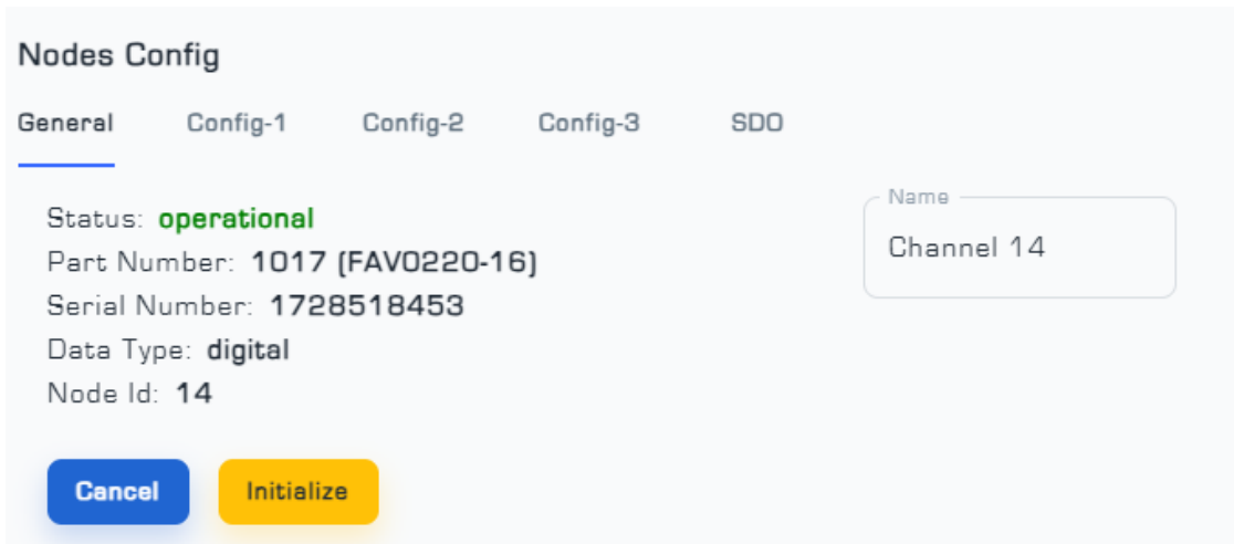
Figure 4: How to Initially Activate a Node
